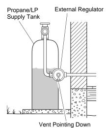
Figure 13 - External Regulator With Vent Pointing Down
